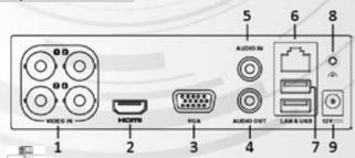
The rear panel of DS-7108HGHI-F1/DS-7116HGHI-F1 provides 8/16 video input interfaces.
